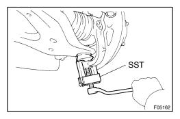
(b) Using SST, disconnect the steering knuckle from the lower suspension arm.
